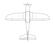
wing span 7.9 m wing area 9.5 m<sup>2</sup>
